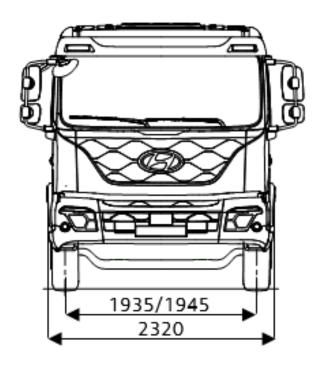
ELWB Wheelbase WB 4900mm OL 8615mm OW 2320mm OH (Standard Roof) 2605mm FOH 1415mm 2300mm Chassis Width 840mm Chassis Height 900mm
