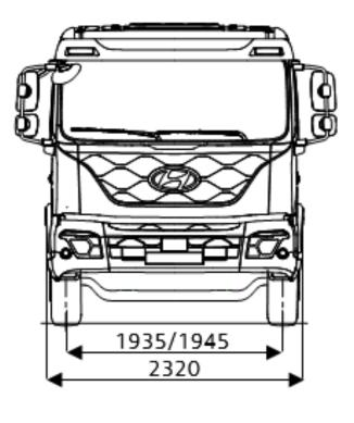
Wheelbase ULWB 5700mm WB OL 8615mm OW 2320mm OH (Standard Roof) 2605mm FOH 1415mm ROH 2650mm Chassis Width 840mm Chassis Height 900mm
